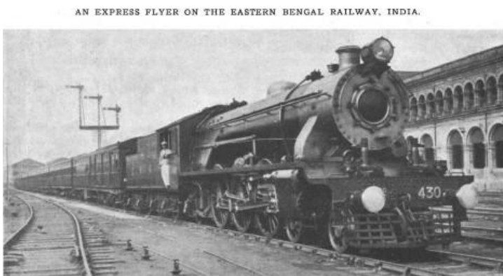
Darjeeling mail train at Sealdah, Calcutta. This train weighs 527 tons, and is hauled by a Class XB engine weighing 155 tons.
